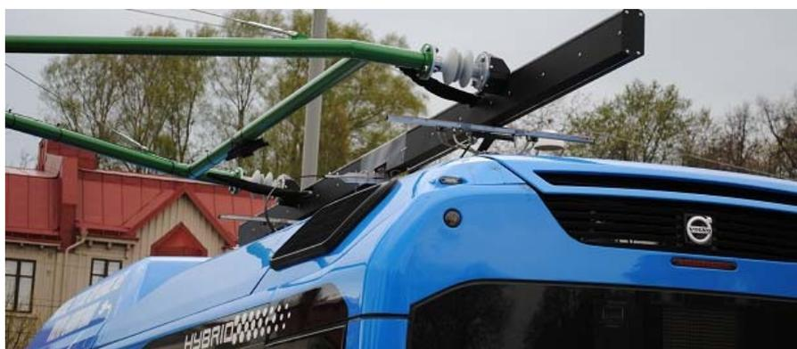
**Figure 2** A VOLVO hybrid bus is being charged at a charging station in Gothenburg
