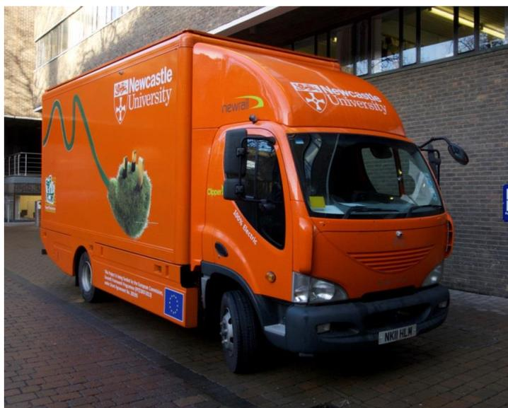
**Figure 10: The Smartfusion Electric Vehicle for last-mile delivery from the consolidation centre to the Newcastle University campus**
