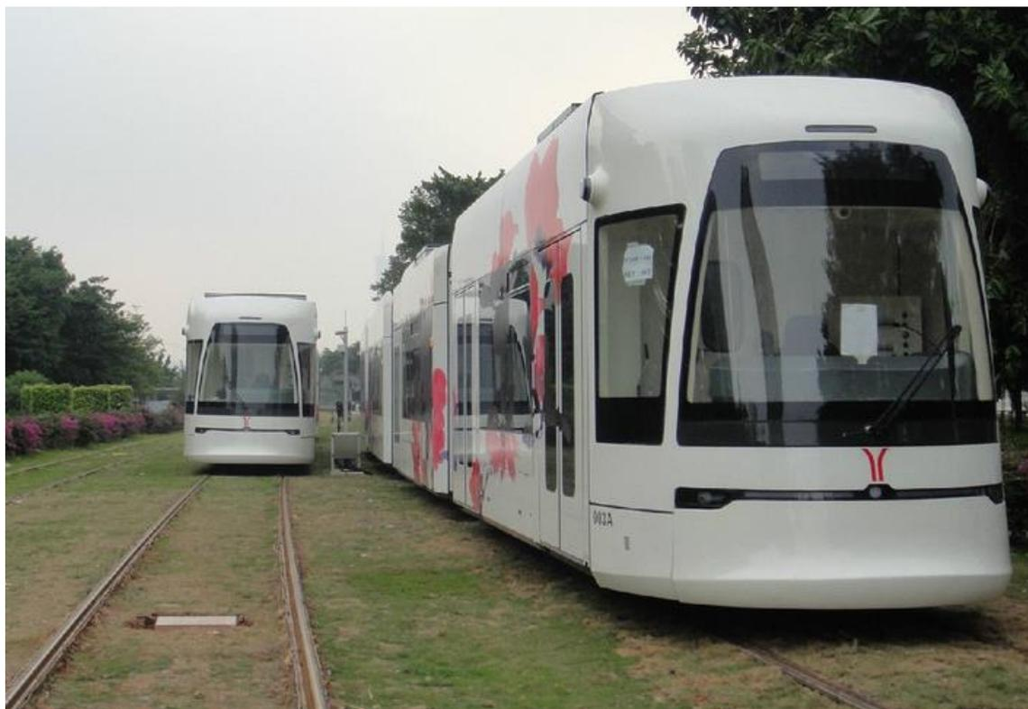
**Figure 4: Two of the seven supercapacitor trams operating on the Haizhu Line**
