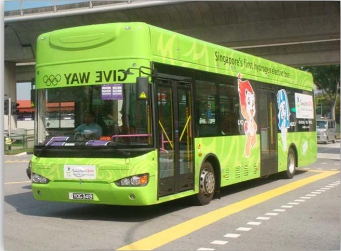
Additionally, the hybrid bus, which runs on both diesel and electricity, was brought in by ComfortDelGro Engineering in collaboration with Shanghai Sunlong Bus Company and Gemilang Coachworks of Malaysia. Fuel savings of up to 30% are derived by using regenerative braking energy stored in on-board lithium-ion batteries to power the bus and hence reduce fuel consumption. The bus uses a parallel hybrid system that is developed by Eaton Corporation of the United States.
