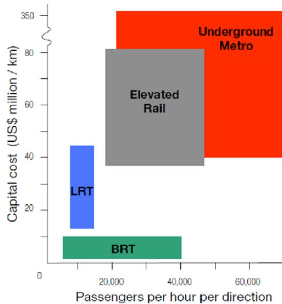
**Figure 7 - Passenger capacity and capital cost for mass transit options, Source: (Wright & Hook, 2007)**
